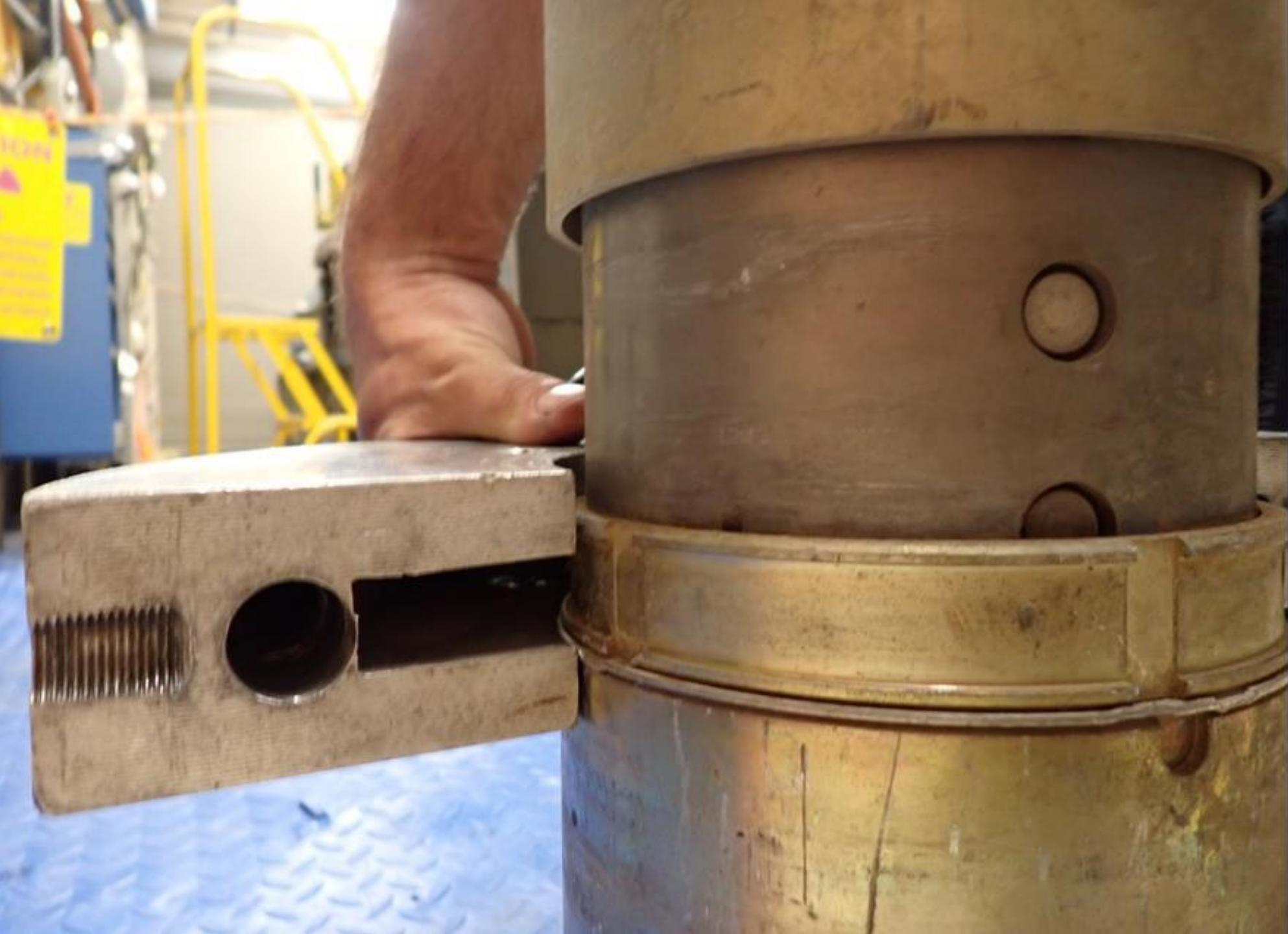
**SLIDE SLEDGE:** A COMMERCIALLY AVAILABLE DEVICE CAPABLE OF KNOCKING OUT SUPPORT PINS WITHOUT THE USE OF A SLEDGEHAMMER AND PUNCH. THIS TOOL COMES IN SEVERAL SIZES AND WITH MULTIPLE AVAILABLE ACCESSORIES. ITS USE CAN HELP KEEP HANDS OUT OF THE LINE OF FIRE THUS BEING A BENEFIT TO PERSONNEL SAFETY.
