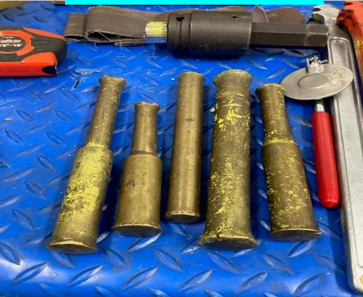
VOGTLE 1-2 NUCLEAR STATION: MECHANICS FABRICATED A DEVICE IN-HOUSE TO ADDRESS A SAFETY ISSUE. WHILE INSTALLING LARGE SNUBBERS ONTO THREADED END TAIL PIECE THE LIFTING AND TURNING OF SNUBBERS SAFELY IS A BIG CHALLENGE. THIS SPINNING TOOL WILL ALLOW LIFTING AND TURNING OF THE SNUBBER ALL IN ONE DEVICE. THE SNUBBER CAN ALSO BE LOCKED IN PLACE WITH SEVERAL BOLTS ALREADY INSTALLED THUS MAKING THIS TASK A LOT EASIER AND SAFER.
